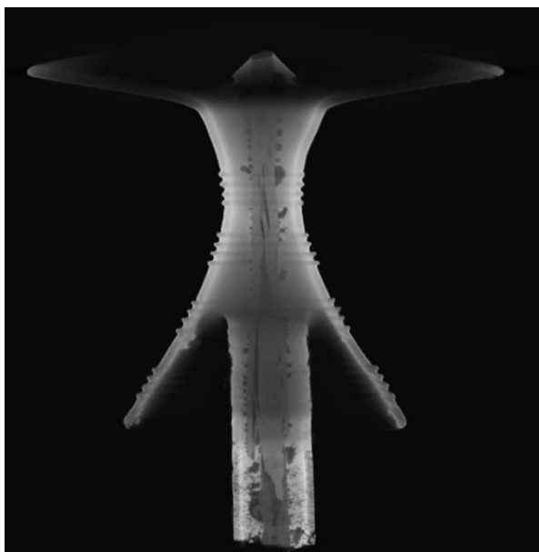
2. Bimetallic pommel and an X-ray \mu CT slice through the object showing an iron tang and casting flaws
