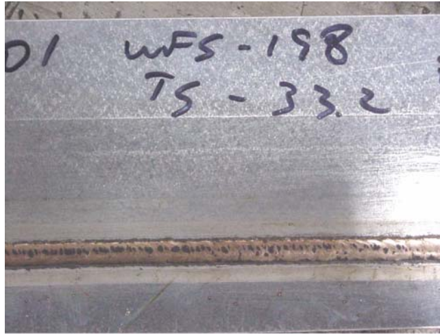
Figure 7. Spatter free GMAW-Pulse braze weld.
