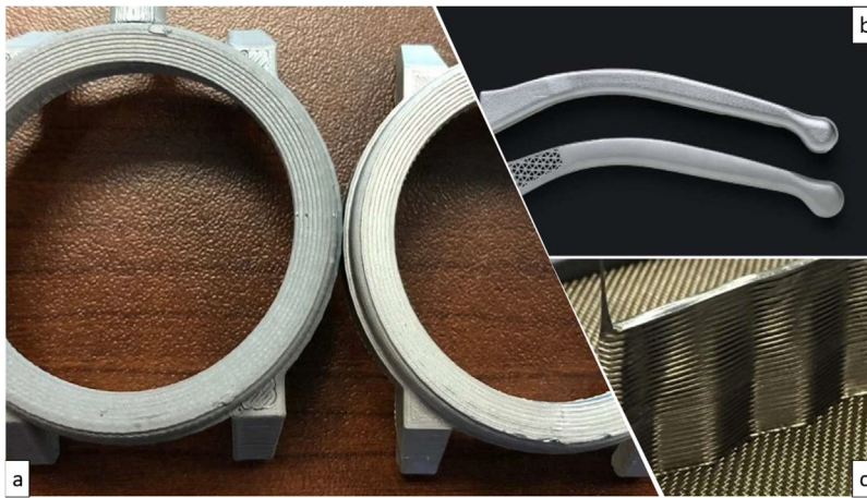
Fig. 9. Functional printed components fabricated using extrusion-based AM of metal/metal-composites: (a) 17-4PH stainless steel, (b) 17-4PH stainless steel (post-processed), and (c) bulk metallic glass (BMG) (adapted from Refs. [66,68,69]).
