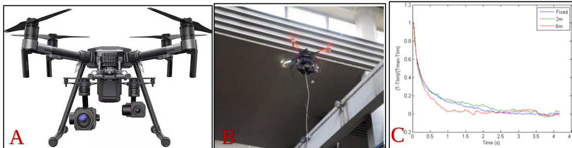
FIGURE 14 A: DJI M210 equipped with thermal camera [8]. FIGURE 14 B: UAV equipped with thermal camera [7]. FIGURE 14 C: Comparison of front face temperature responses to flash heating in the case of a large uniform irradiation with a fixed camera and a stabilized camera with UAV at two distances (2 m and 6 m) [7].
