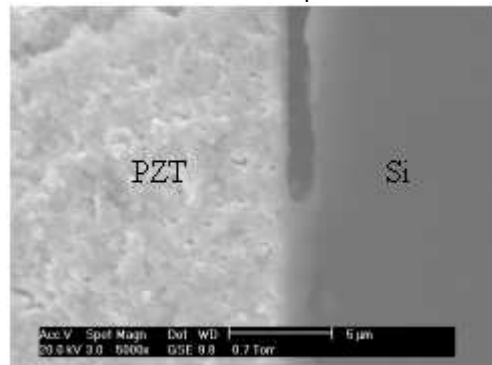
Fig 2. Holes produced at the Si/PZT interface due to diffusion of the Pb into the Si substrate during sintering.
