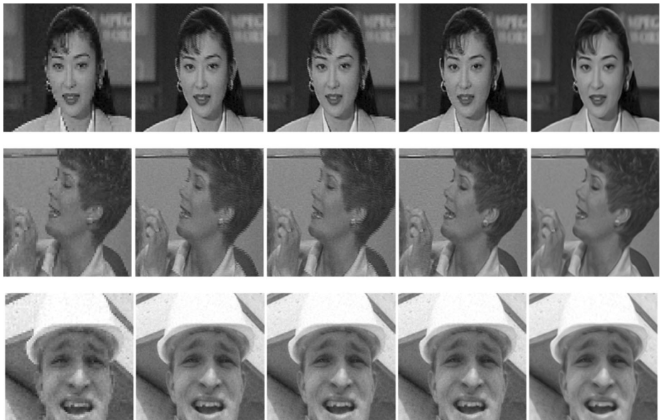
Fig. 4 Results of produced HR images using different SR methods for a randomly selected frame of Akiyo , Mother & daughter , and Foreman video sequence respectively. Column 1: input LR frame, Column 2: Bicubic, Column 3: Vandwalle-SANC, Column 4: Keren-SANC, and Column 5: the proposed technique
