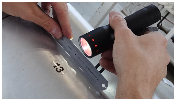
Figure 1.8: The use of a flashlight may help to highlight the gap between surface and ruler.
