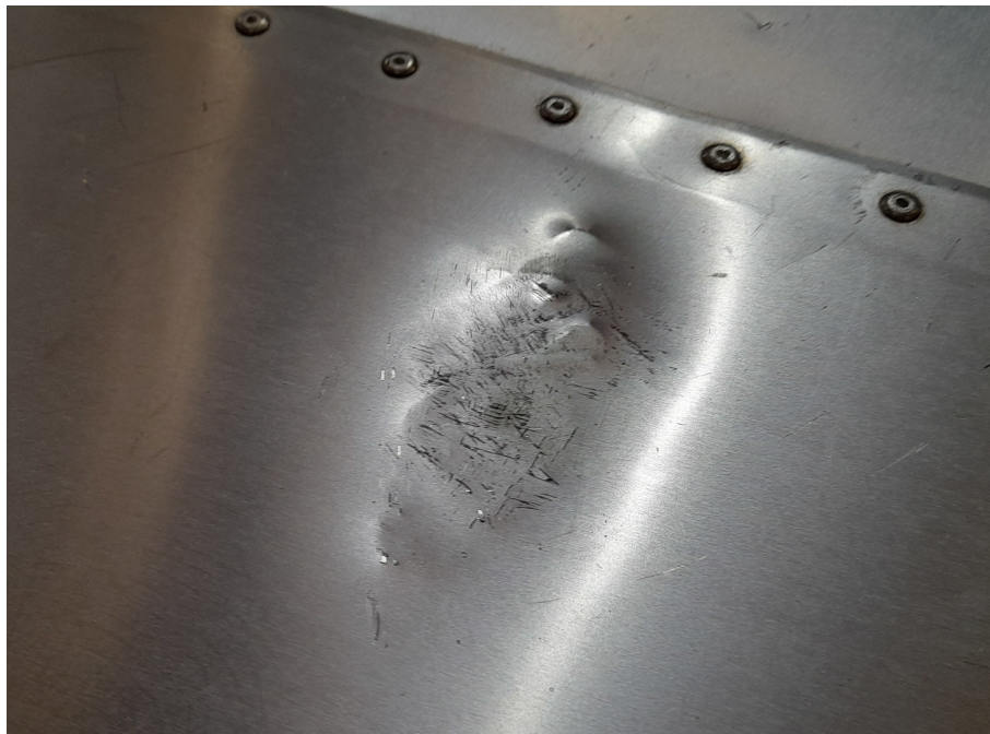
Figure 7.2: Detail of the dent on the Eurostar rudder.
