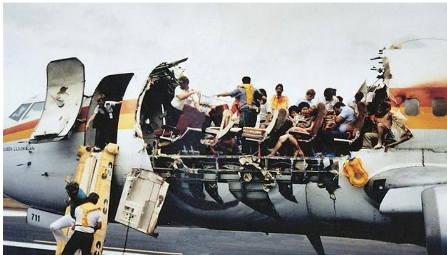
Figure 1.4: The Aloha accident: the B737-200 lost its upper part due to undetected damage. A flight attendant lost her life and several people were injured.
