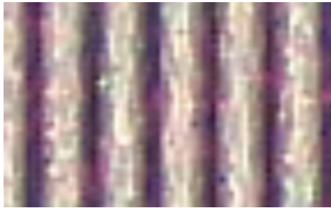
(a) Detail of a fringe pattern projected by a class 1 laser projector.
