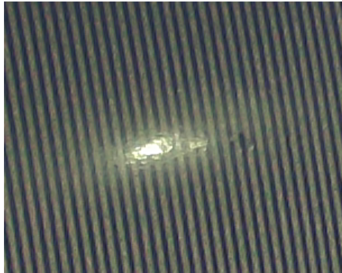
Figure 7.13: Reflection over Cranfield B737-400 fuselage. Detail of the projected pattern that becomes unreadable in the reflection area.
