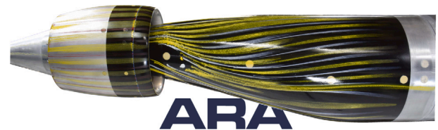
Fig. 11. Photograph of an oil flow visualisation around the tail of a novel aircraft wind-tunnel model, courtesy of ARA.
