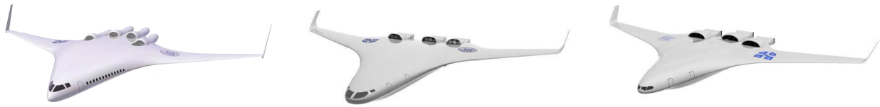
Fig. 28. Main conceptual aircraft designs generations: SAX-12, SAX-20, SAX-40. Source: Retrieved from Ref. [133].
