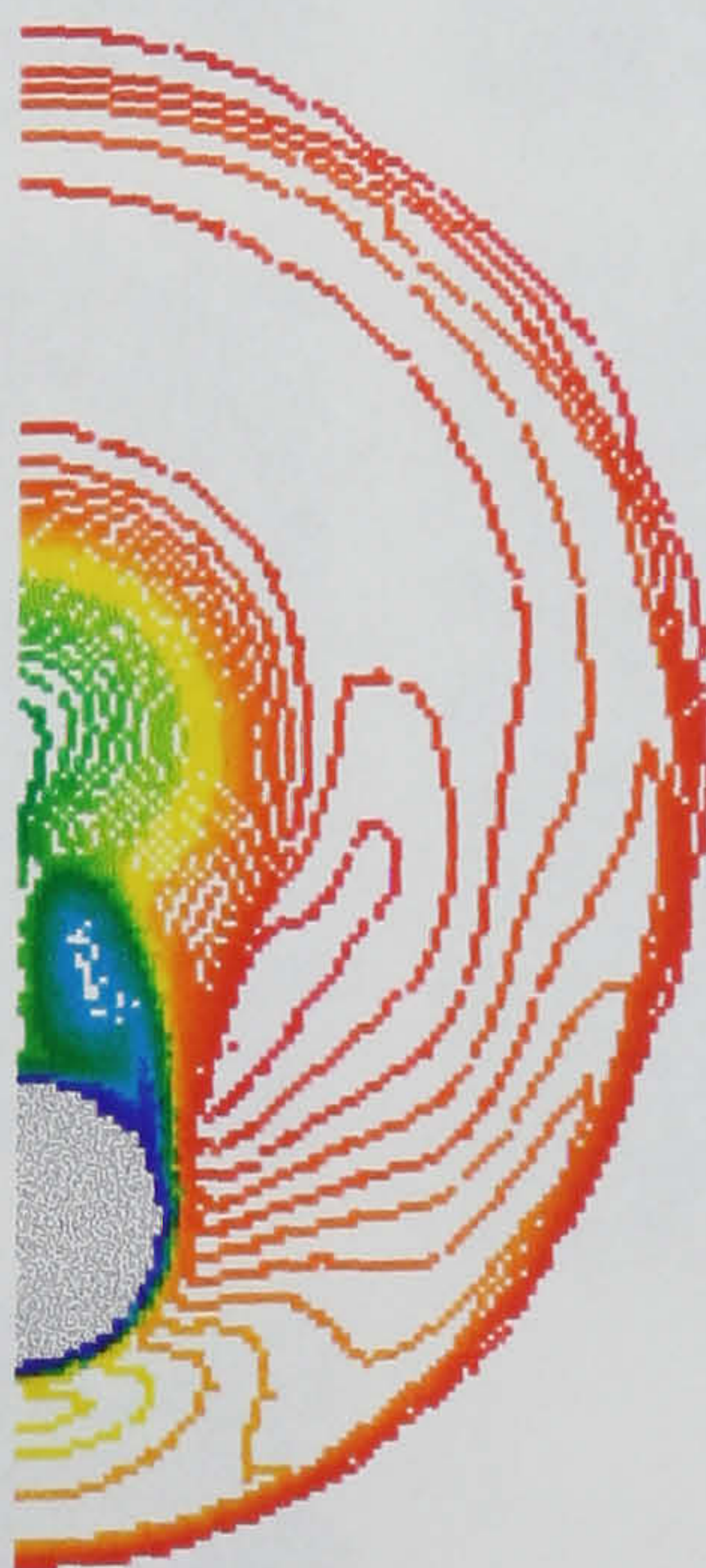
(e) Mach number contours in the cross-flow plane at the cone-cylinder base
