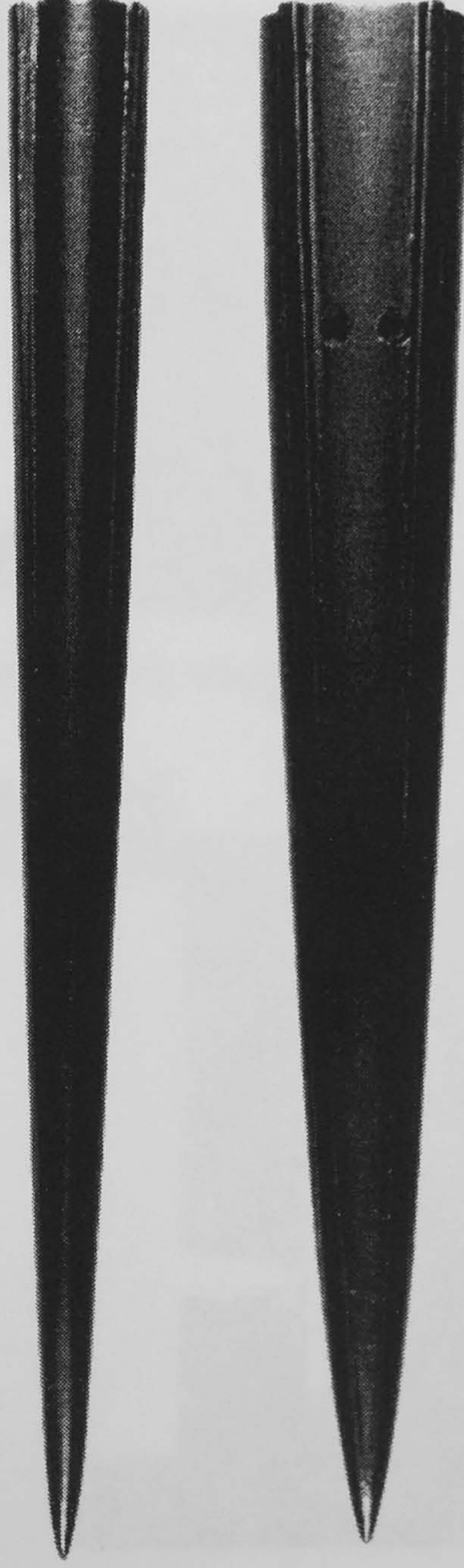
Top and side view of the power-law body with strakes
