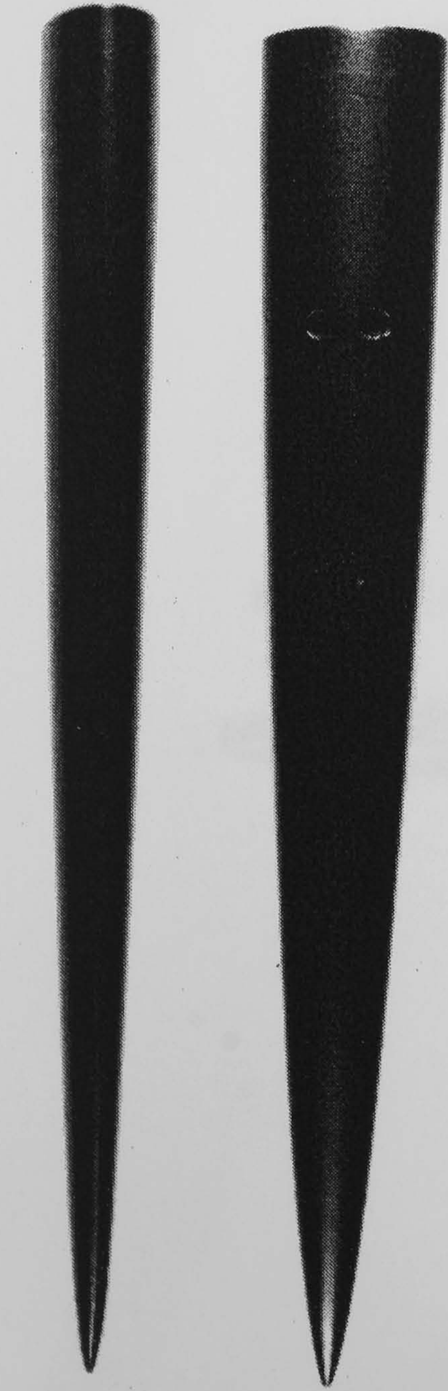
Top and side view of the power-law body without strakes
