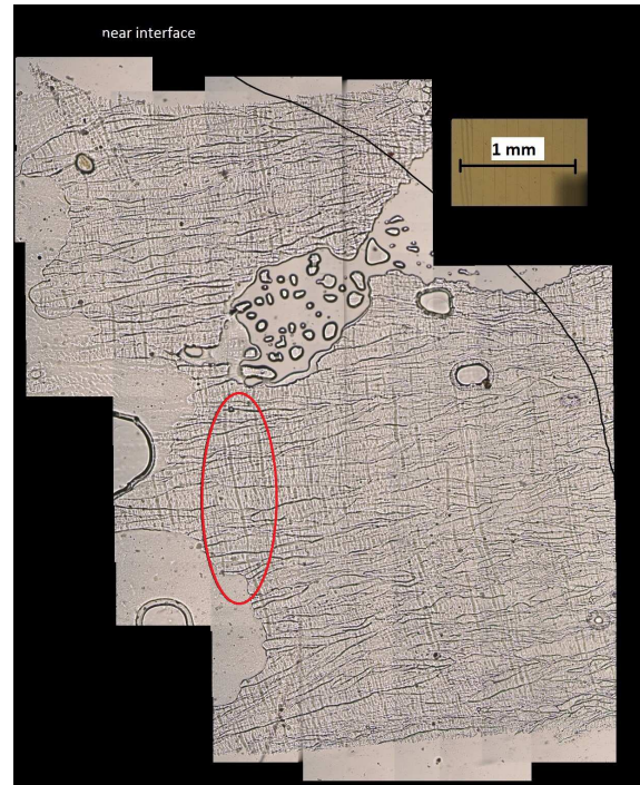
Figure 7: Microstructure of the longitudinal cut of ice built on a mirror polished surface finish titanium alloy substrate ( T=-15^{\circ}\text{C} , \text{LWC}=0.3 \text{ g.m}^{-3} , V=80 \text{ m.s}^{-1} , \text{MVD}=20 \mu\text{m} )
