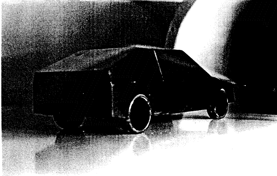
Figure 4 . 1 a Smoke Flow Visualization for the Basic Saloon (Square-Edged Fastback Configuration at 10 Degrees Yaw)
