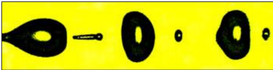
Figure 159: Droplet image obtained from strobe illumination with low-power LED
