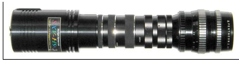
Figure 66: Astronomy camera with Extension Tubes and 135mm Lens.
