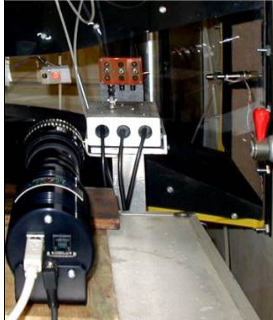
Figure 67: Wind tunnel test with prototype LED flash and Astronomy camera.
