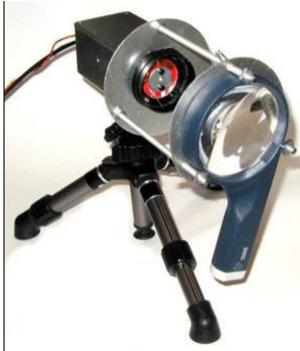
Figure 171: LED flash unit with Collimating Lens
