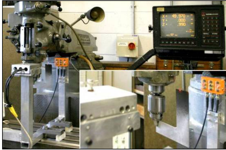
Figure 150: Alignment of diode lasers on milling machine bed
