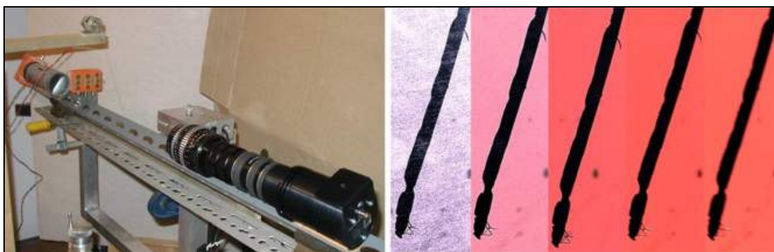
Figure 164: Test of LED flash unit and camera with resulting images at 100m/s.
