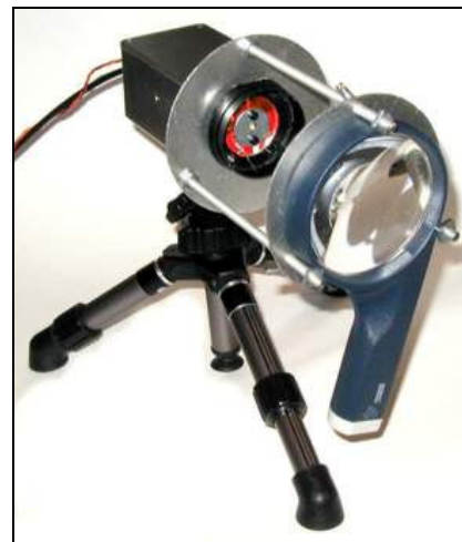
Figure 11: LED flash unit with 80mm Collimating Lens
