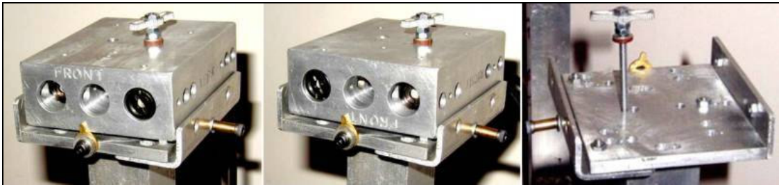
Figure 151: Arrangement for supporting and inverting the diode laser block.
