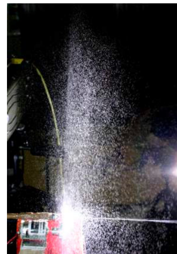
Figure 143: Testing of spinning disc droplet generator.
