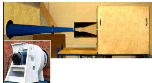
Figure 10: Convergent Droplet Tunnel with Plenum chamber, Diffuser and Fan
