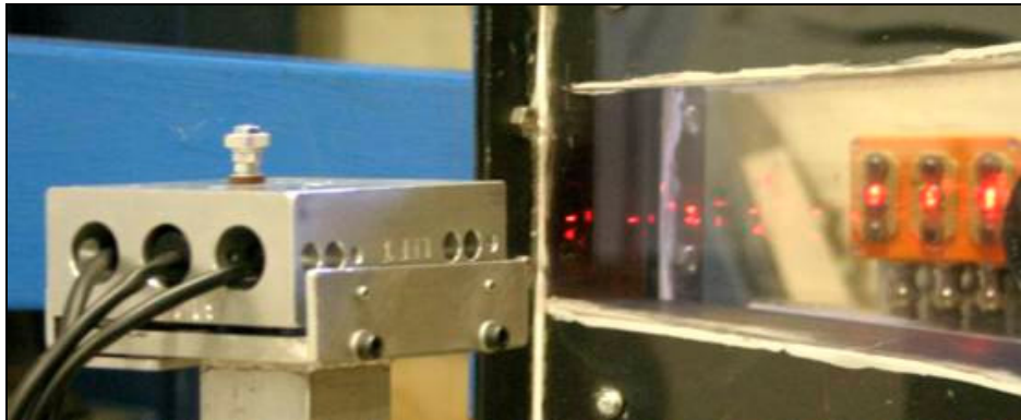
Figure 79: Close-up view of the laser beam block and photo detectors
