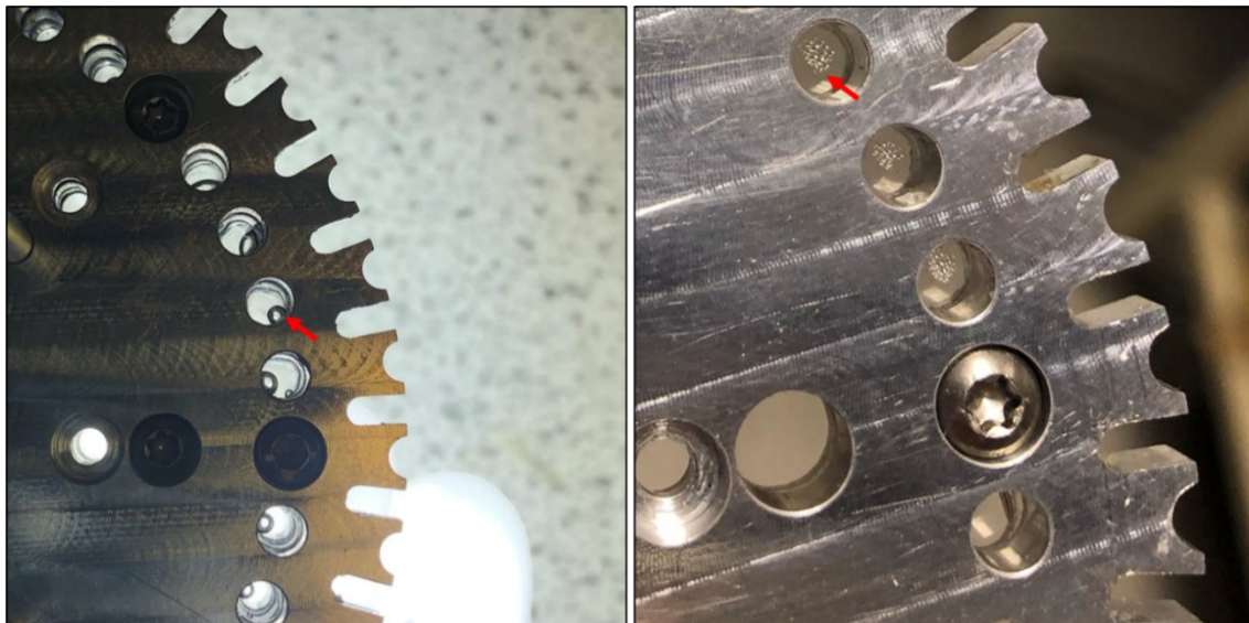
Figure 3-21. Example of images with bubble and condensation formation on the MCSD.
