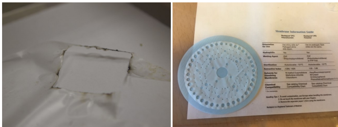
Figure 3-8. Left – CO 2 laser cut polycarbonate. Right – UV laser cut polycarbonate.
