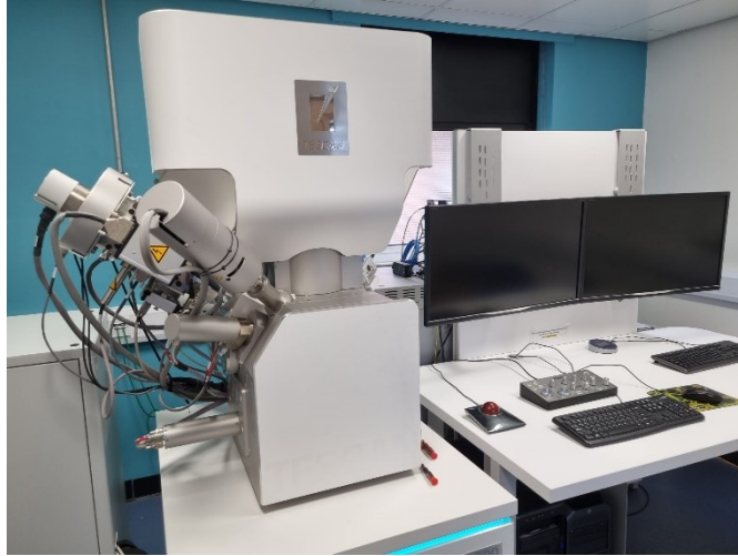
Figure 3-9 The S8215G field emission SEM utilised in this work.
