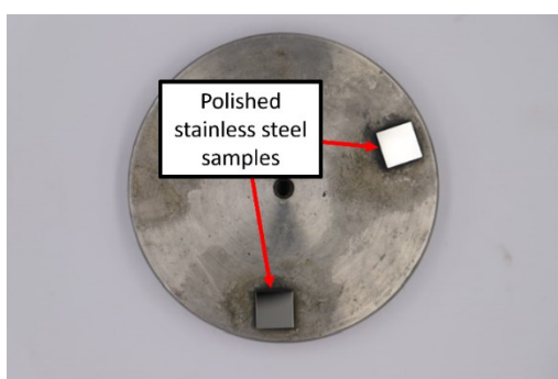
Figure 3-1 Polished stainless steel samples used for SPL and FIB prototyping.
