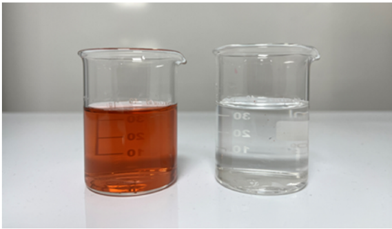
Fig. 12. Image of bioleaching solution before (left) and after (right) metals recovery by electrowinning and precipitation.
