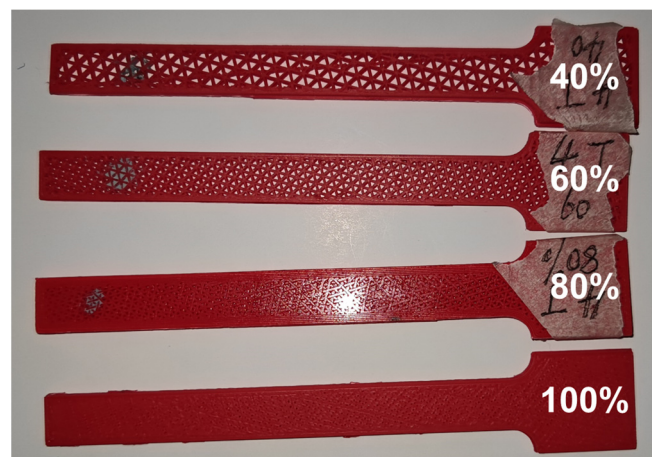
Figure 12. The specimens with different infill densities (0.4 mm nozzle size and triangle pattern).
