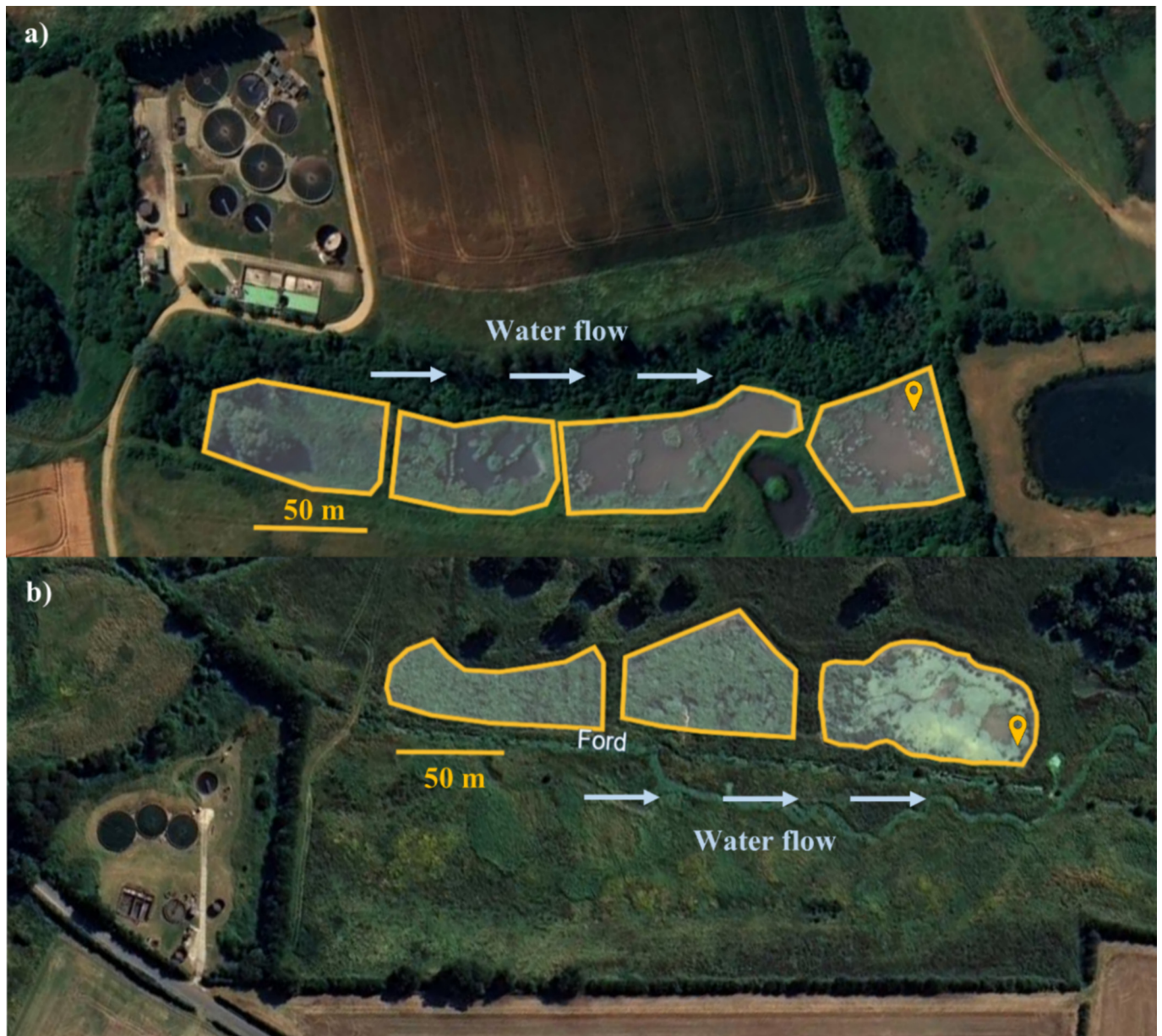
Fig. 1. Aerial views of Ingoldisthorpe (a) and Langham (b) treatment wetlands. Yellow lines outline the boundaries of each cell in the systems. The yellow map pointer marks the outlet of the final cell in each wetland and the light blue arrows indicate the water flow direction.
