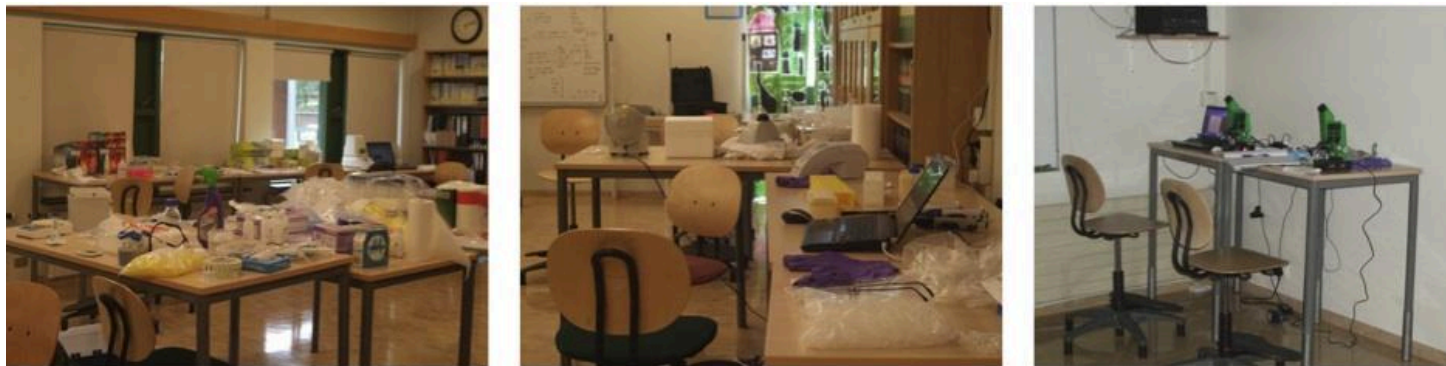
Figure 7 - The three workstations as set up in our field laboratory. (l) DNA extraction, purification, and qPCR area, with general supply table in foreground. (c) ATP bioluminescence area, with FM staining area in the background. (r) 'Darkroom' established for fluorescence microscopy.
