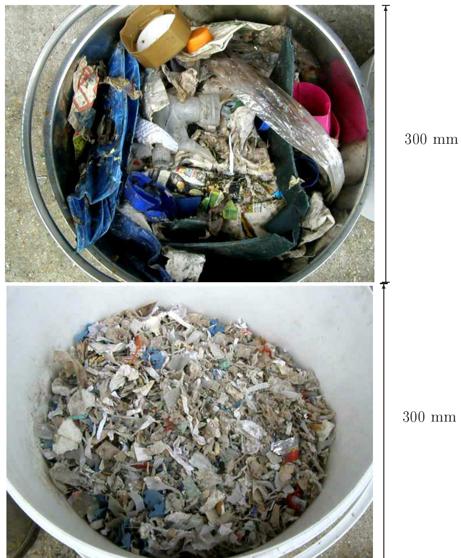
Figure 4.2: Comminution of MRFR. Photographs shows selected material before and after size reduction using the laboratory cutting mill.
