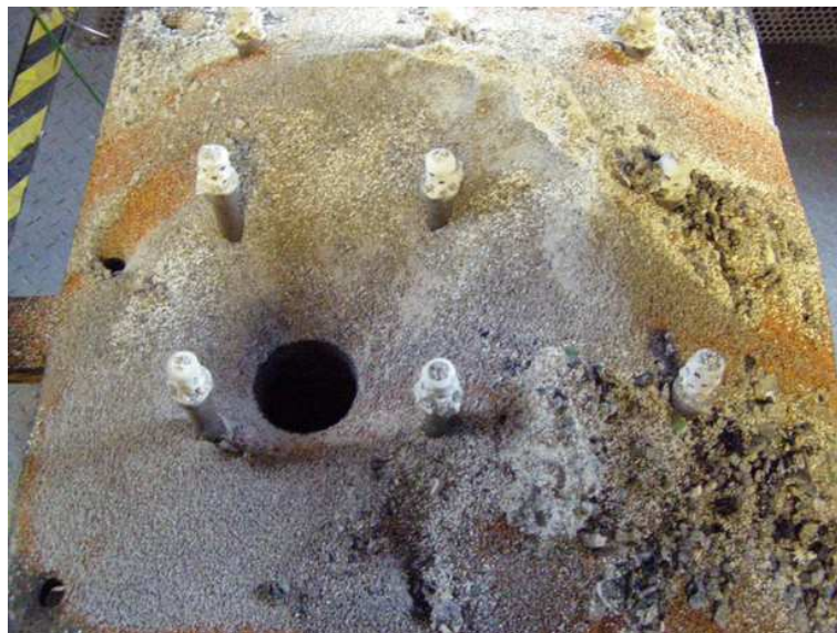
Figure E.3: Agglomeration of fluidised bed material during combustion of DDGS-MRFR (90:10). The hole is the drain as shown in Figure 3.4
