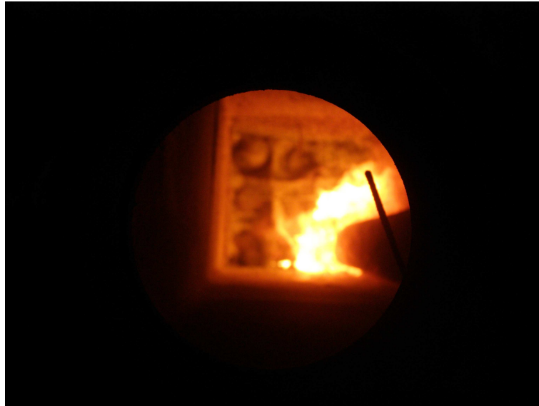
Figure E.1: De-fluidisation of fluidised bed material during combustion of DDGS-MRFR (90:10); appearance of the fluidised bed from above (viewing downwards), using the inspection hole at the top of the combustor. Circular areas of fluidised bed material correspond to areas immediately above the gas distribution grid nozzles where air flow was able to agitate the granules, to maintain fluidisation. The areas appearing as lines correspond to static areas of defluidisation where the fluidised bed material was stationary, i.e. where agglomeration had occurred.
