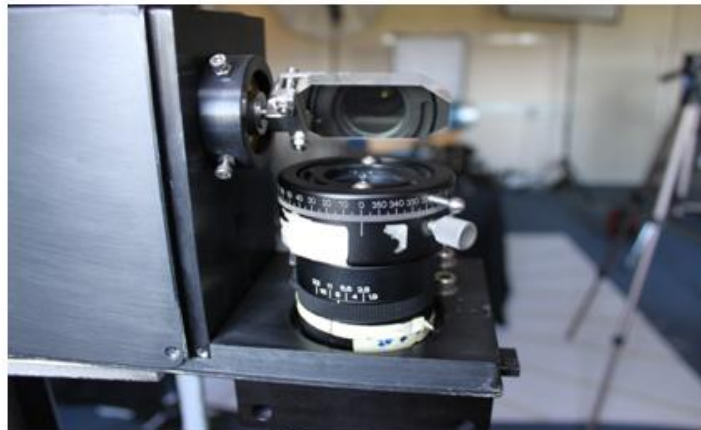
Figure 4 The polarizer is placed on the camera lens.
