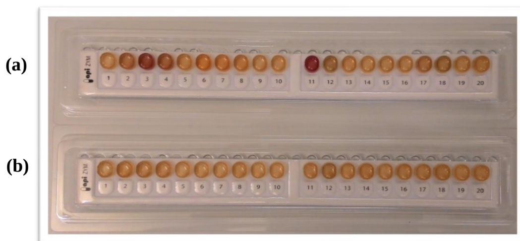
Figure 4.1 API ZYM strips showing enzymatic activity (colour changes and intensity) for 19 different enzymes in the supernatant of T. rubrum grown on SBD broth at (a) 0.99 a_w and (b) 0.95 a_w for five days at 30°C.
