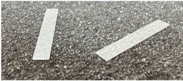
Fig. 2. BGO slices used for micromachining tests.
