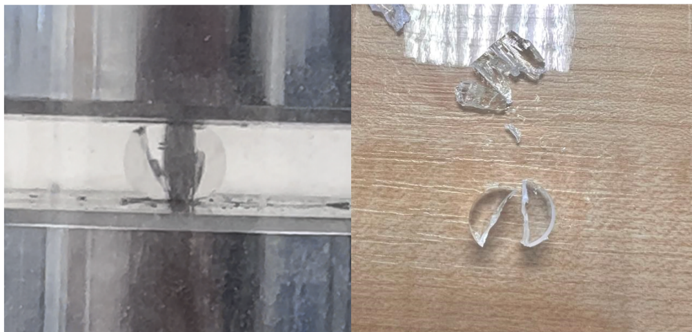
(e) Real failure of material.
