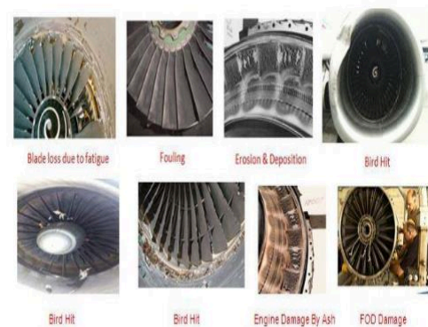
Figure 8 Types of Gas Turbine Faults
