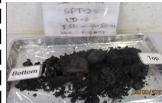
Fig. 5. Photos of retrieved waste samples: (a) as-excavated samples; (b) oven-dried and sieved samples; (c) borehole samples from Cell N; (d) borehole samples from Cell S.
