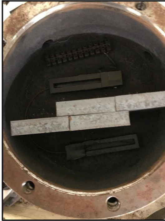
Figure 79: Metal plates placed between propellant trays to prevent ignition before PIC.
