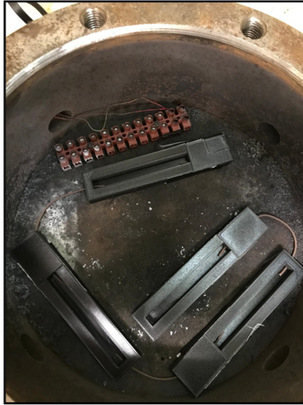
Figure 78: 20 Grams of propellant divided into 4 equal trays of 5 grams.
