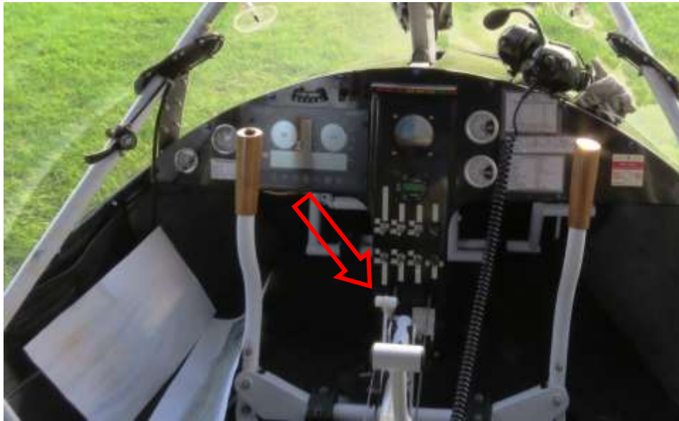
Figure 10. Location of the pitch trim control lever in a Raj Hamsa X'Air cockpit (lever nearer camera is a throttle, black lever on left hand cockpit frame is an engine choke control).
