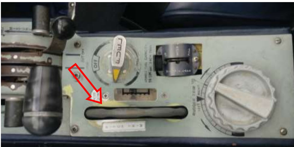
Figure 2. Pitch trim wheel in the Bulldog (located between the seats, front of aircraft is to the left of the image, wheel on right of image is yaw trimmer)
