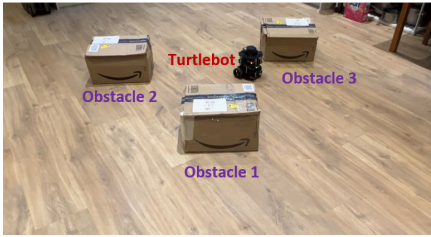
Fig. 8: Real-world testing environment of the Turtlebot with three random static obstacles.
