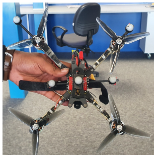
Figure 6: Symmetrical Structure - SY.
