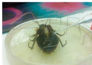
Figure 2.8 Using cockroach as a biofuel-cell [30].
