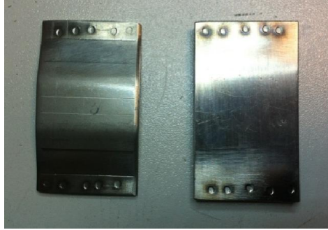
Figure 5.12 Resistance welded endcap.
