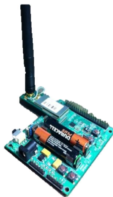
Figure 5.27 Jennic Ltd wireless integrated transceiver compliant with IEEE 802.15.4 protocol at 2.4GHz frequency.
