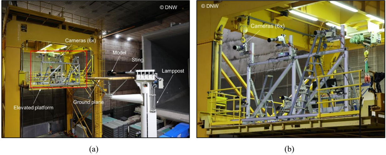
Fig. 4 (a) Photograph of the test set-up and elevated platform with the camera frame; (b) close-up view of the six PIV cameras mounted on the platform.
