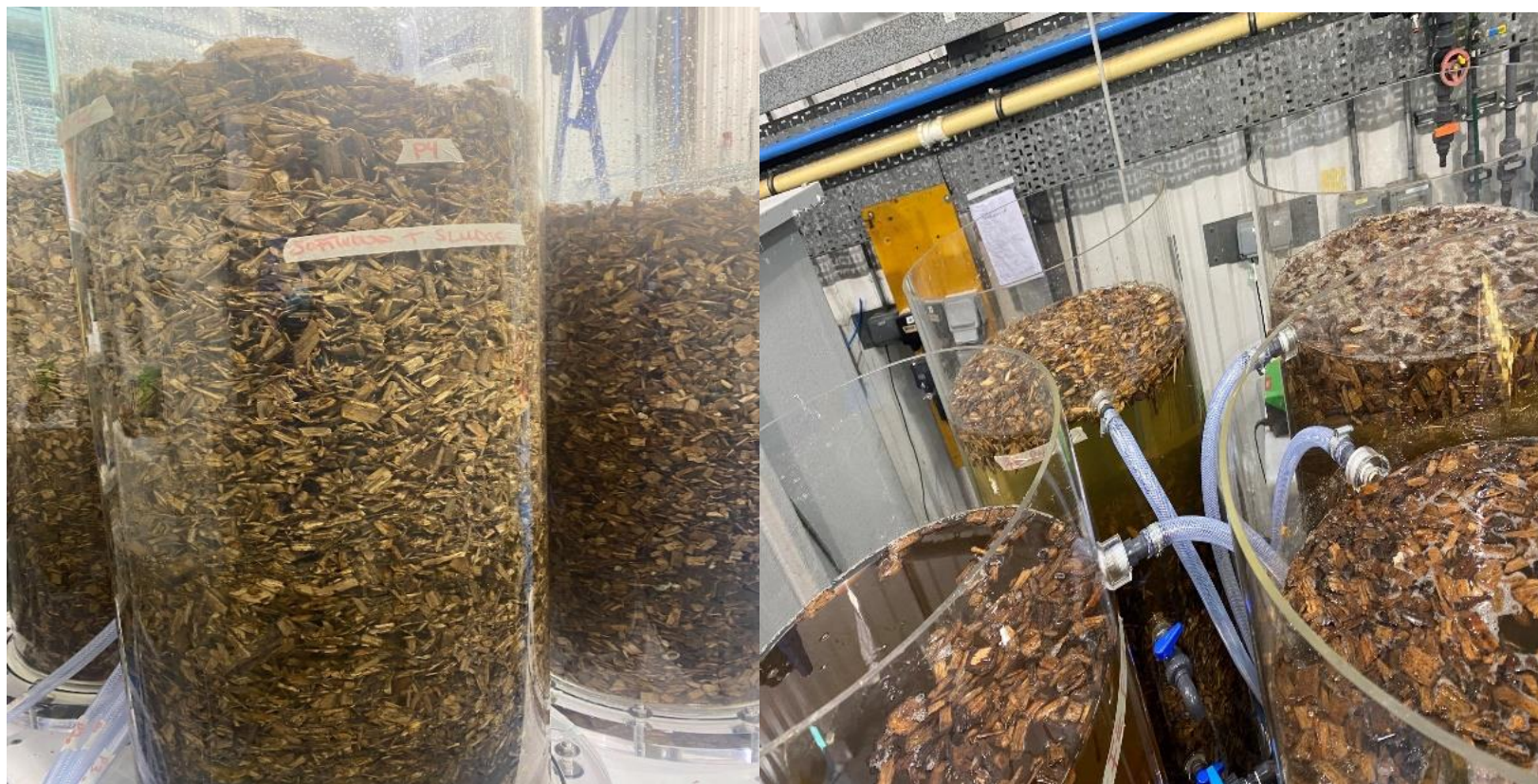
Figure A-2 Column media before and after effluent flow
