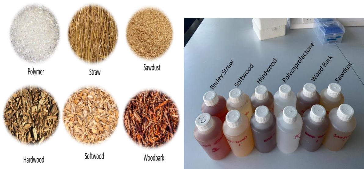
Figure 3.1 Leaching tests done on variety of solid organic media.
