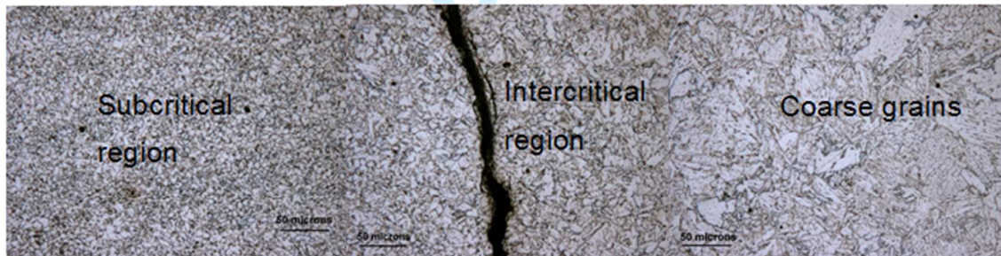
Figure 17 Crack growth in the Intergranular HAZ region (X5)
