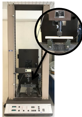
Figure 3 Hounsfield MOR machine setup
