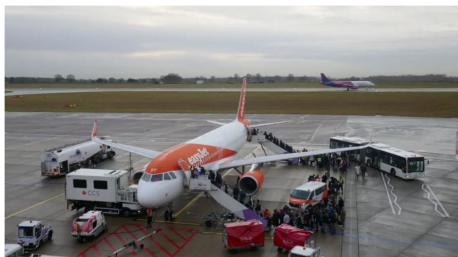
Figure 2. Ground support equipment and vehicles servicing aircraft.
