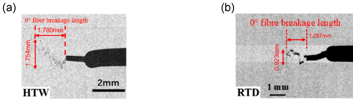
Fig. 4. Typical CT images of 0° plies at (a) HTW and (b) RTD [18] conditions. Note. The saturated damage height at HTW and RTD condition are 1.754 mm and 0.923 mm, respectively.
