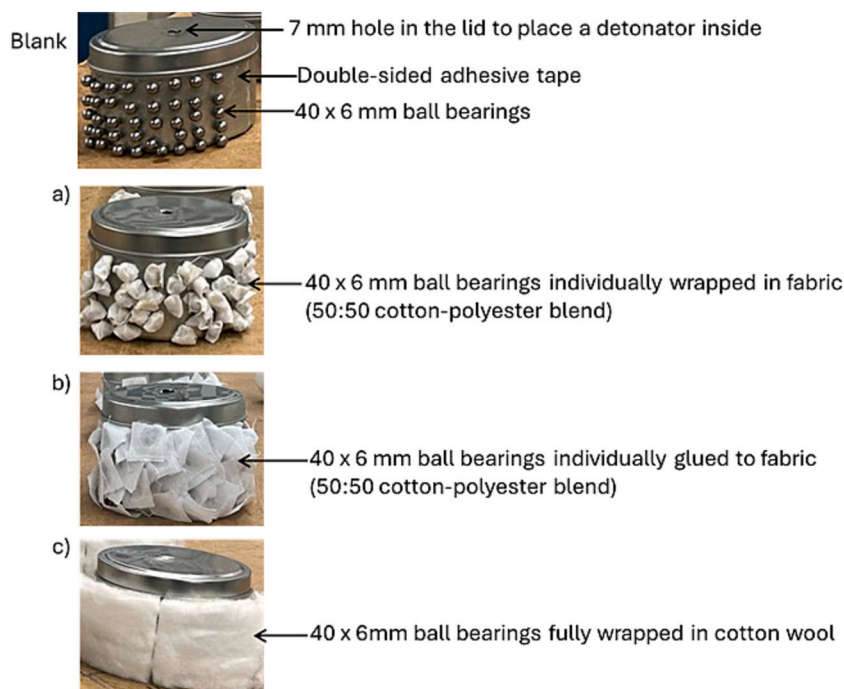
Fig. 3. Diagram of all three deposition methods and blank IED.
