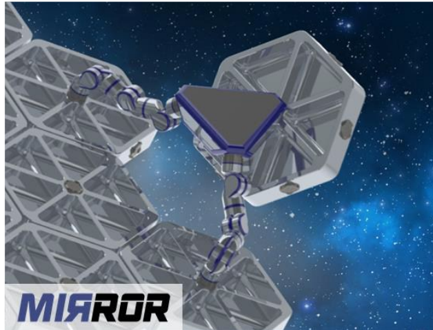
Figure 2: Multi-Arm Robot (MAR) for on-orbit large telescope [16]
