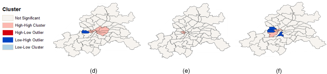
Fig. 14. Hot spot analysis of the estimation's error by the end of the training - d) ANN autoregressive e) ANN multivariable, f) Bass model.
