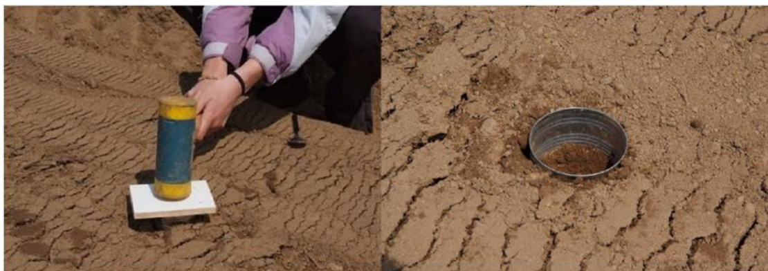
Figure 3.5 Soil sampling procedure (a) driving cylindrical steel sleeve into planting bed; (b) sleeve with upper layer of soil removed. Diameter of core = 4 cm.
