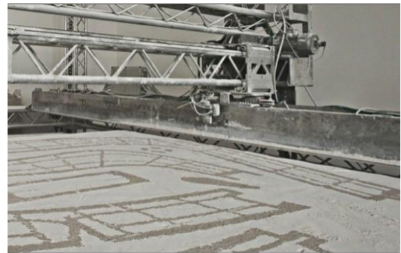
Figure 8. D-Shape printing technology (Monolite UK (Dinitech SpA), 2016).
