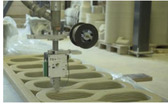
Figure 7. Material extrusion system (Paolini et al. , 2019).
