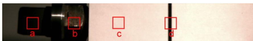
Figure 14. Image with and without white sheet paper. The squares a and b enclose different parts of the accelerometer and the squares c and d contain locations of the white paper with and without the black straight line. [61].
