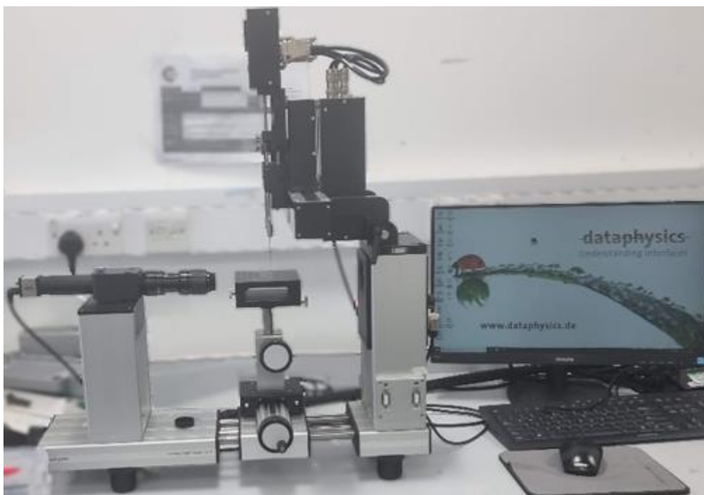
Figure 3-22 OCA 50 by Data Physics Instruments GmbH used to measure liquid contact angles.
