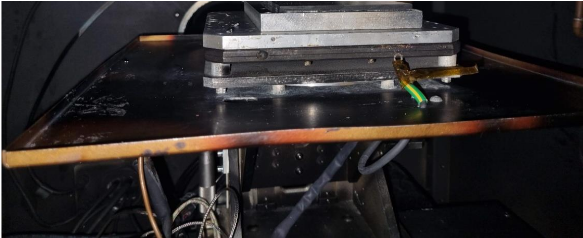
Figure 3-9 Precision motion stage used to pass samples under the plasma torch for both RF, MW and DBD plasma systems.
