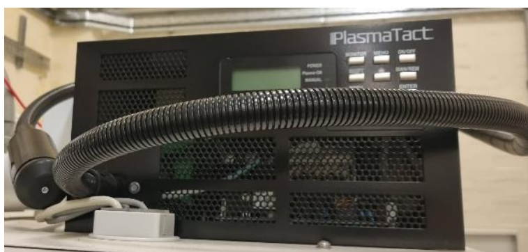
Figure 3-5 front face of the Plasma Tact 50W Microwave induced power plasma system
