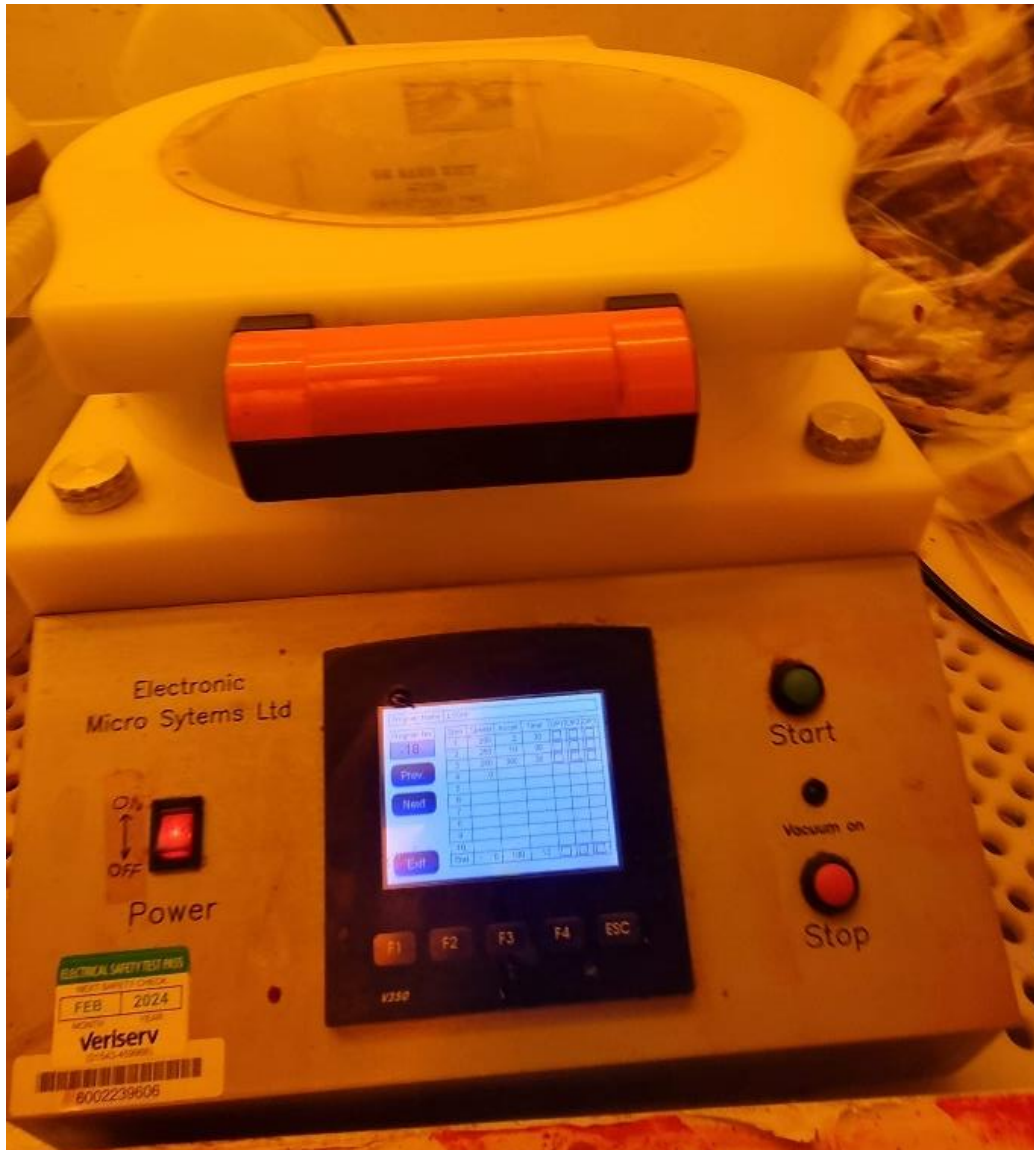
Figure 3-1 Spin Coater used for CM2
