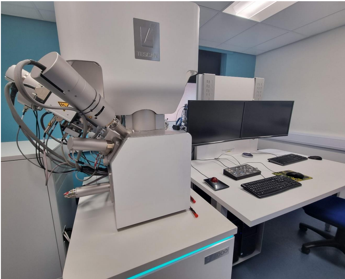
Figure 3-21 featuring a TESCAN S8000 FIB-SEM with attachment capability for FIB and ToF-SIMS.
