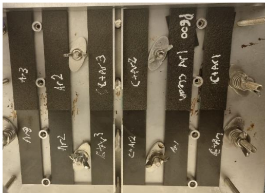
Figure 3-25 showing composite lap shear samples placed on a precision rig, prior to bonding.
