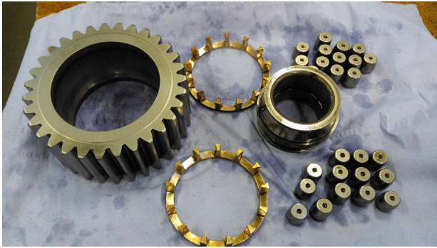
Fig. 6. The components of 2nd planetary bearing.
