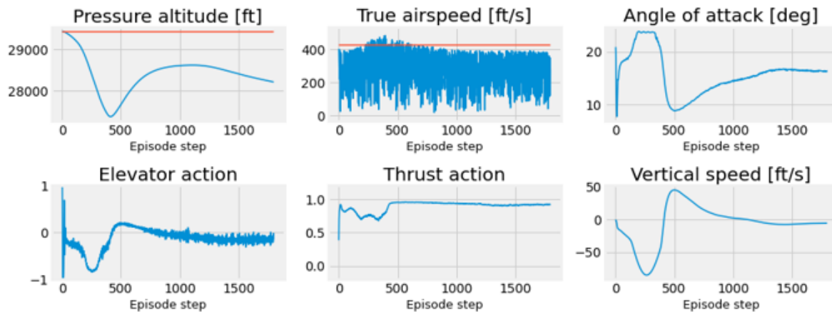
Figure 2. Stall recovery at 29000 ft of the baseline agent trained with a restrictive approach. Random Pitot blockages were included. The altitude and airspeed targets are shown in red.
