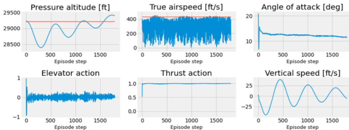
Figure 3. Stall recovery of the baseline agent with more strict termination conditions. Random Pitot blockages were included. The altitude and airspeed targets are shown in red.
