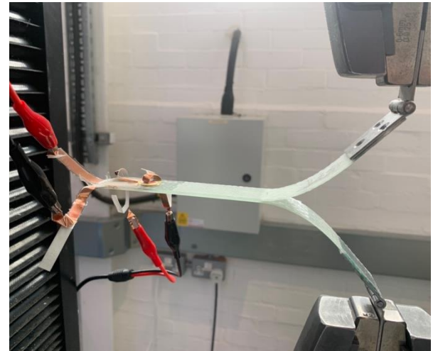
Figure 4-1. The test setup used for (left) three-point bend testing (right) DCB testing
