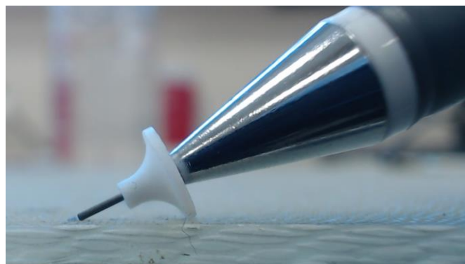
Figure 1-6. The pencil lead-breaking method.
