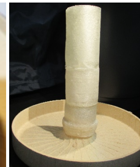
155mm igniter tube with black powder
