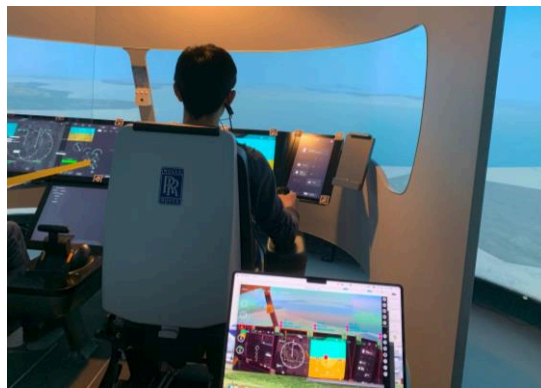
Fig. 3. Participant performing the landing task in the FSS while wearing the eye tracker.
