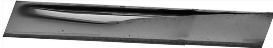
(d) Experimental Bubble shape for EXP4; 160cP oil, Vso = 0.21m/s, VOLgas = 0.001498m 3
