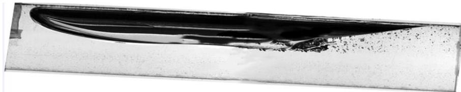
(a) Bubble shape from experiment, EXP2: \text{VOL}_{\text{gas}} = 0.002996\text{m}^3 , L_b = 0.47\text{m} , Fr = 0.4394
