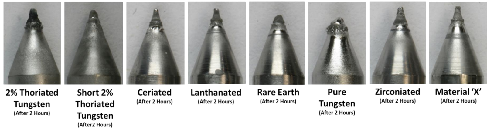
Figure 201 PTA electrode wear and TEAR shape for a standard 2% thoriated tungsten electrode, a special short electrode and seven different materials. Photographed after one hour (top row) and after two hours (bottom row).
