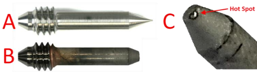
Figure 219 Effect of electrode length on arc starting: A] A new 2% thoriated electrode, B] Reduced electrode length at the point of failure to arc start. C] Close-up of electrode flat tip ‘B’, and evidence of an arc starting cathode spot on flat tip edge.
