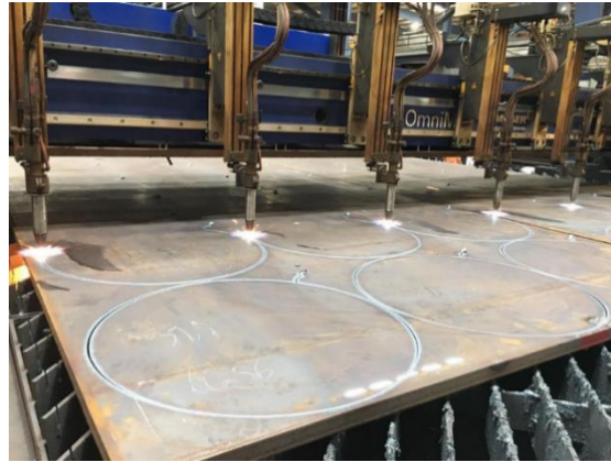
Figure 3 Plasma cutting steel plate and material wastage. Image courtesy of AncoferWaldram steel plates B.V.
