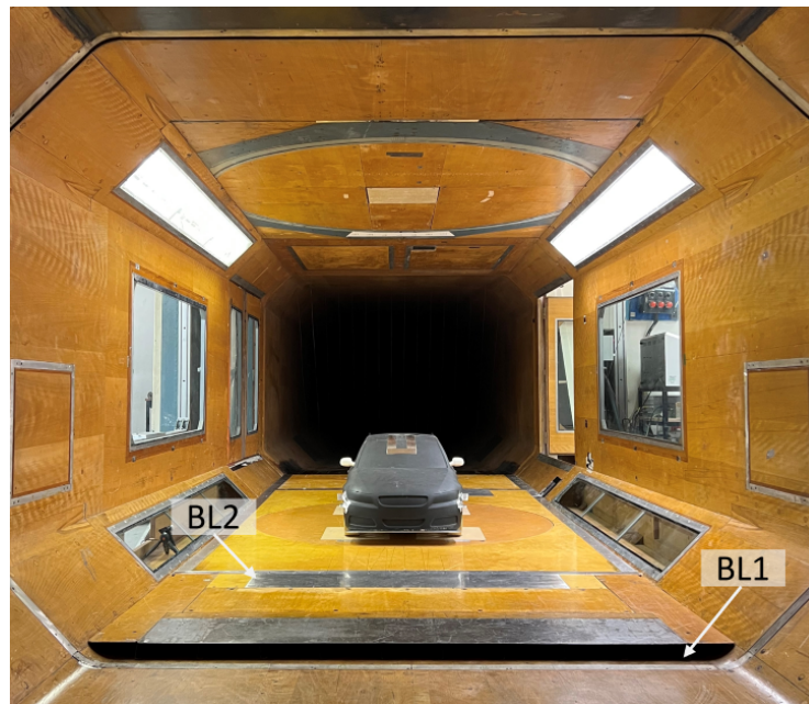
Figure 4.2: Experimental setup in the 8x6 Wind Tunnel at Cranfield University.
